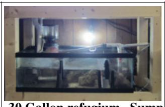
30 Gallon refugium -Sump System includes optional automatic water top off
